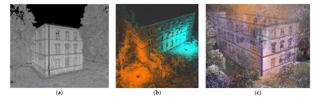
**Figure 6.** (a) Display of laser scanner measuring points Leica BLK 360; (b) Presentation of the laser scanning model; (c) Cyclone Register model.
