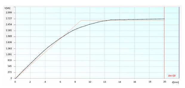
Figure 17. Capacity curve (black) and its bilinear idealization (orange) for y-direction.
