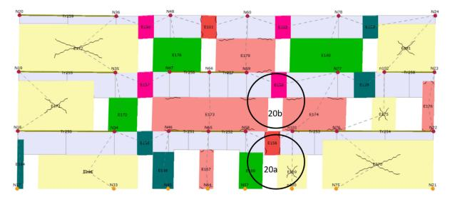
Figure 19. Damage to the central wall in the *x*-direction (3Muri).
