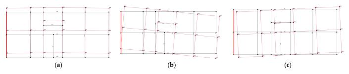
Figure 14. (a) First mode; (b) second mode; (c) third mode.
