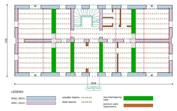
**Figure 22.** Proposal for the position of the new load-bearing walls and proposal for the removal and replacement of partition walls.
