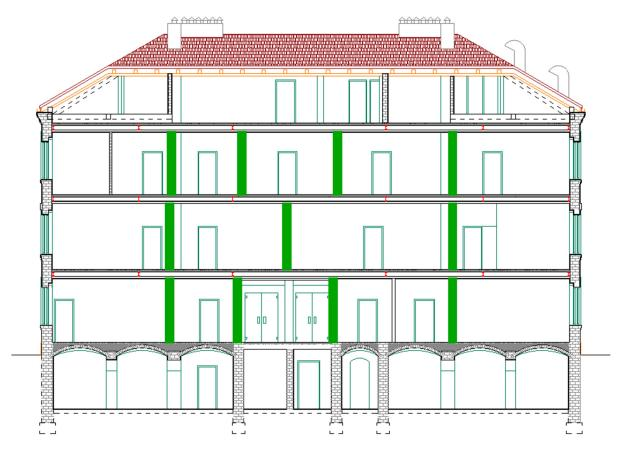
**Figure 23.** Proposal for the position of the new load-bearing walls and proposal for the removal and replacement of partition walls (cross-section).
