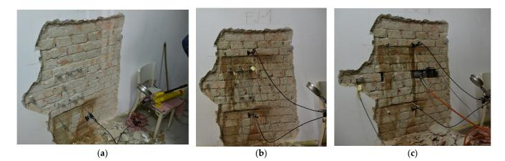
**Figure 10.** (**a**) Connected hydraulic system and flat jack; (**b**) Determination of stress and deformation dependence of masonry; (**c**) Testing of shear strength of masonry with control of vertical stress by flat jacks. (photo credit: Luka Lulić).
