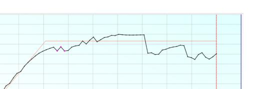
**Figure 16.** Capacity curve (black) and its bilinear idealization (orange) for *x*-direction.
